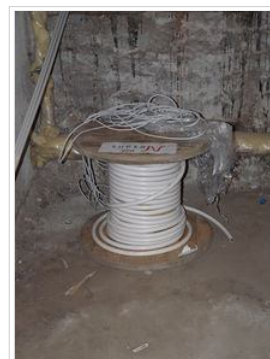
Three-phase copper cable TN-S 16mm 2 with PVC insulation
