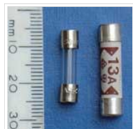
20 mm 200 mA glass cartridge fuse used inside equipment and 1 inch 13 A ceramic British plug fuse.
