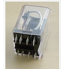
A DPDT AC coil relay with "ice cube" packaging
