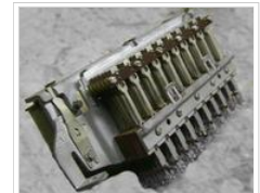
A large relay with two coils and many sets of contacts, used in an old telephone switching system.
